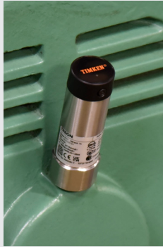
Wireless sensor installed in equipment
