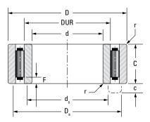
ADAPT bearings are interchangeable with ISO toroidal and spherical roller bearings.
