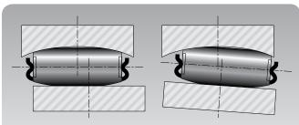
The design of the ADAPT bearing allows for simultaneous axial float and a misalignment capacity of 0.5 degrees. The rollers align with the inner ring regardless of axial displacement and misalignment.
