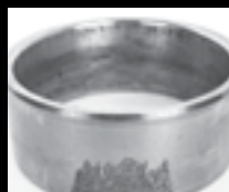
Geometric Stress Concentration (GSC) spalling on inner ring
