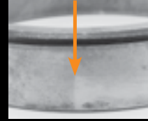
Witness mark from high spot in the housing
