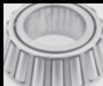
Fracture on inner ring
