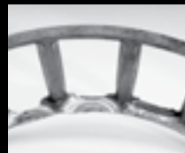
Cage pocket wear from excessive roller movement
