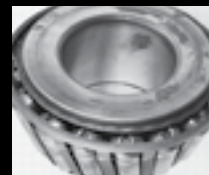
Scoring damage on roller end
