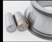
Fine particle contamination
