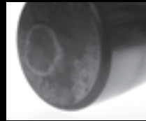
Roller end with adhesive wear
