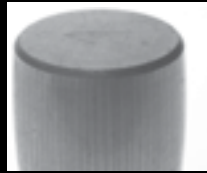
Fluting caused by electric current
