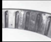
Heavy false brinell on outer race
