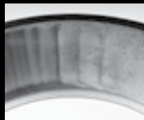
Scalloping marks in the cup caused by excessive endplay
