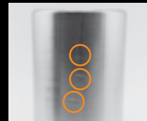
Nicks and dents caused by rough handling
