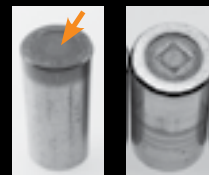
Rib and roller end heat damage
