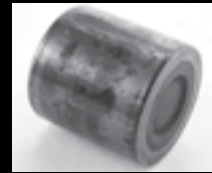
Roller flats, adhesive and skidding wear on raceway surface
