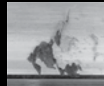
Point Surface Origin (PSO) spalling
