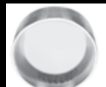
Elliptical roller path caused by misalignment
