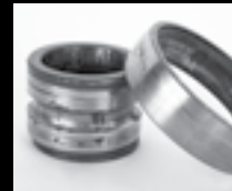
Advanced corrosion and etching
