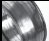
Adhesive wear on bearing inner ring
