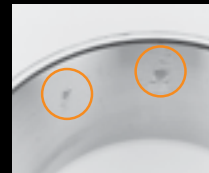
Roller spaced nicking
