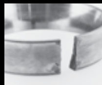
Loose fit resulting in stretched and broken cup
