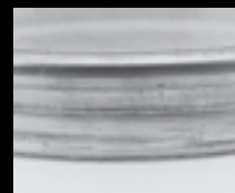
Loose outer ring fit in a wheel hub
