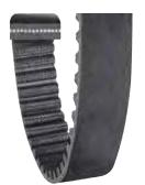
The Panther XT high torque synchronous belt is a powerful alternative to chain or a drop-in replacement for polyurethane belts. Carbon cord construction and abrasion resistant tooth fabric contribute to longer belt life and reduced maintenance, downtime and noise levels.
