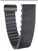
ACHE belts are designed for air-cooled heat exchangers. The belt is built with only "Z" twist cords. This gives the belt an upward direction that helps keep the belt off the bottom flanges, reducing excessive wear on the bottom side of the belt.
