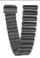
Proven performance from both sides of the belt for greater flexibility and efficiency in your drive design. Unitized process joins top and bottom teeth into one homogeneous belt with 100% rated capacity on both top and bottom side of the belt. Full fabric facing is included on all teeth.
