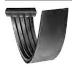
Wedge-Band Chipper Drive belts are specially designed and constructed to meet the unique demands of the forestry industry. It's designed to slip during "overload" or drive stall conditions. By allowing the belt to have controlled slippage, less heat is generated, which results in longer belt life.
