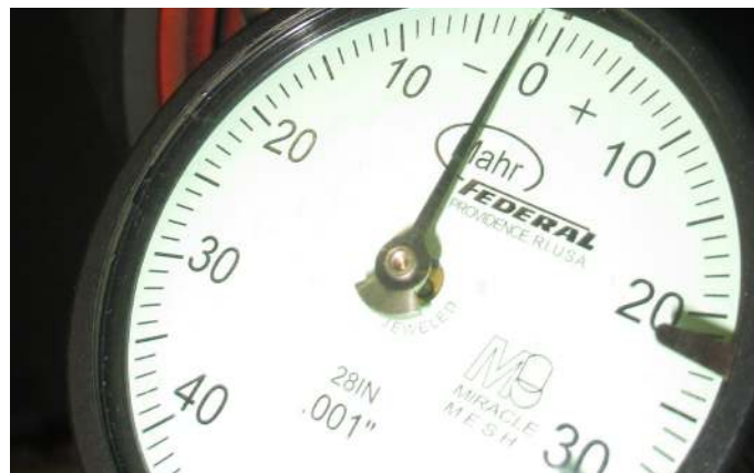
Fig. 12. The bearing lateral endplay should be 0.001 in. to 0.015 in. (Amtrak 0.001 in. to 0.020 in.).
