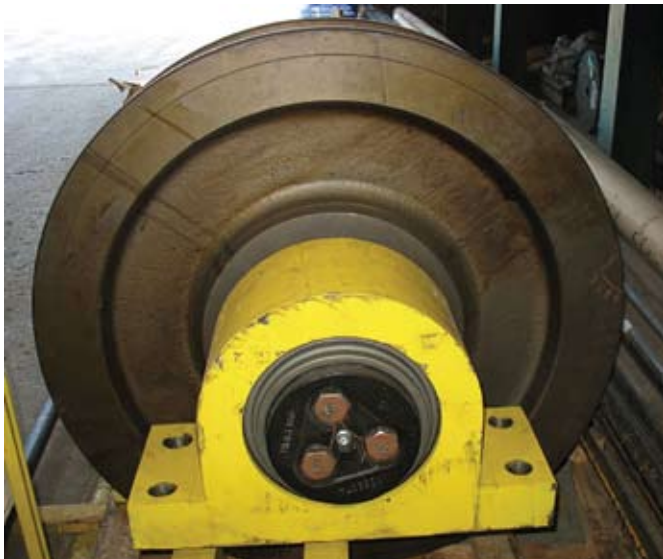
Fig. 12 AP bearings used in pillow block application
