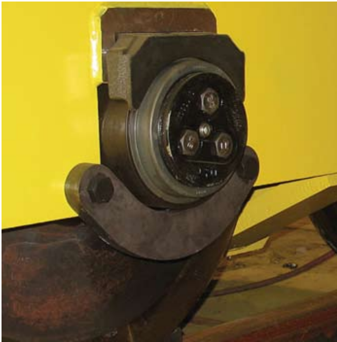
Fig. 8 Narrow adapter mounting on trolley safety bar
