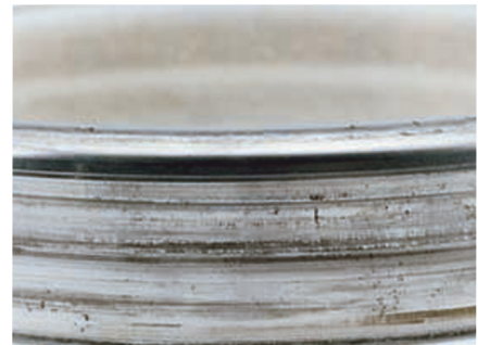
Bearing cup (outer race) damage caused by an excessively loose fit in a rotating hub.
