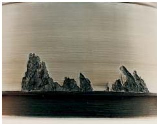
Geometric stress concentration (GSC): Misalignment, system deflections and heavy loading.
