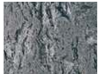
Full race width fatigue spalling: Caused by heavy loads creating a thin lubricant film and elevated temperatures.
