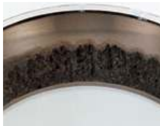
Irregular roller path from deflection, inaccurate machining or wear of bearing seats.
