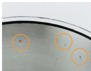
Roller spaced nicking: Raised metal on races from contact with roller edges.
