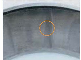
Scalloping: Uneven localized wear resulting from excessive end play.
