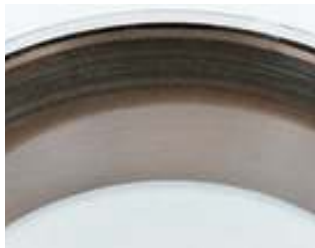
Irregular roller path from deflection, inaccurate machining or wear of bearing seats.
