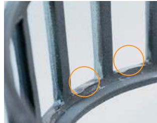
Cage pocket wear: Heavy contact between rollers and cage pocket surfaces caused by bearing operating too loosely.
