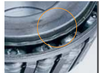
Bearing cone (inner race) large rib face deformation: Metal flow from excessive heat generation.
