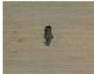
Inclusion origin: Oxides or other hard inclusions in bearing steel.
