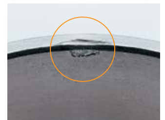
Bearing cup (outer race) face denting: Indentations from hardened driver.
