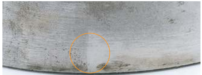
Localized spalling on the bearing cup (outer race) from stress riser created by split housing pinch point.
