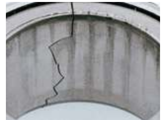
Bearing cone (inner race) bore damage: Fractured cone due to out-of-round or oversized shaft.
