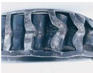
Total bearing lock-up: Rollers skew and slide sideways.
