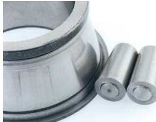
Abrasive wear: Fine abrasive particle contamination.
