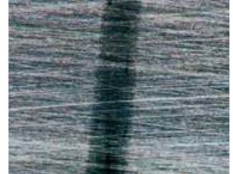
Damage from shock or impact.
