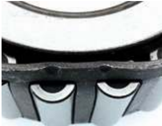
Cage deformation: Improperly installed or dropped bearing.
