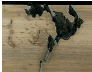
Point surface origin (PSO): Debris and raised metal exceeding the lubricant film thickness.
