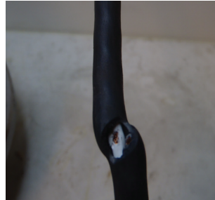
Avoid pinched cable by using retainer clips.
