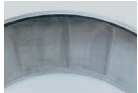
Fig. 1 - Outer race (cup) scalloping; uneven localized wear resulting from excessive end play.
