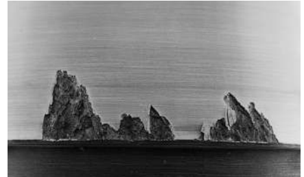
Fig. 2: Geometric Stress Concentration (GSC) spalling
