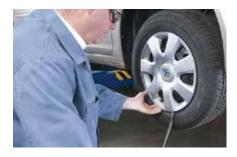
Raise the vehicle. Remove the wheel cover to access the lug nuts if needed. Remove the lug nuts and the wheel.
