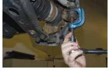
5. Remove the upper tie rod using the proper tool.
