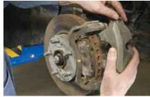
Remove the caliper and the caliper mounting bracket.
