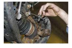
If present, disconnect the ABS sensor wire from its mating connector point and secure the sensor cable to prevent damage.
