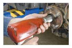
Remove the axle nut using an axle nut socket.
