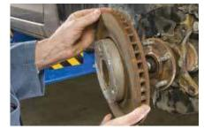
3. Remove the brake rotor. Follow the vehicle manufacturer's recommendations for rotor inspection and reuse.
