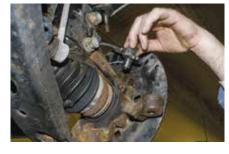
6. If present, disconnect the ABS sensor wire from its mating connector point and secure the sensor cable to prevent damage.
