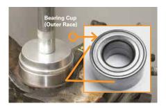
Press the new bearing into the steering knuckle using an appropriate press and support fixture. The outside diameter of the tooling surface must be large enough to support the bearing cup (outer race) of the bearing assembly.
