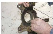
Clean the steering knuckle of debris or burrs using a fine file, wire brush, emery cloth or honing stone. Inspect the bearing contact surfaces for wear and burrs.
