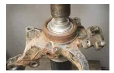
Remove the bearing from the steering knuckle using an appropriate press and support fixture.
