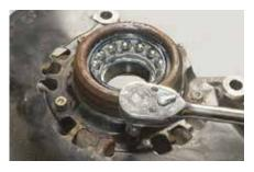
3. Remove the disk brake dust cover.
