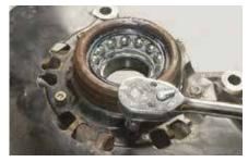
3. Remove the disk brake dust cover.
