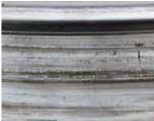
Bearing cup (outer race) spinning: Loose cup fit in a rotating wheel hub.
