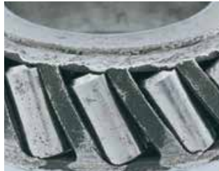
Rollers binding and skewing: Cage ring compressed or interfered with during installation or service.
