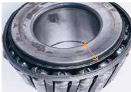
Fig. 11: Tapered roller bearing cone large rib face deformation, caused by metal flow from excessive heat.
