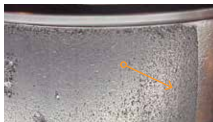
Figs. 14 & 15: Peeling: Micro-spalling in a tapered roller bearing outer race (above) and inner race (below) due to thin lubricant film from elevated temperature.
