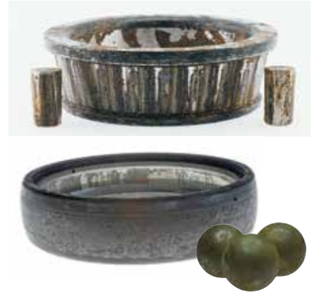
Figs. 16 & 17: Etching: A tapered roller bearing cone and rollers and a ball bearing outer race and balls show rusting with pitting and corrosion from moisture/water exposure.
