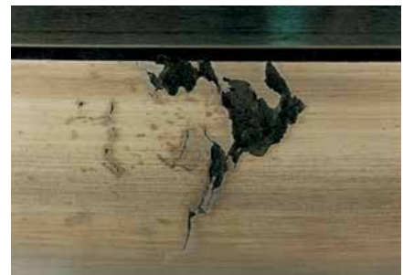
Fig. 19: A tapered roller bearing inner race (cone) with spalling from debris contamination bruises.
