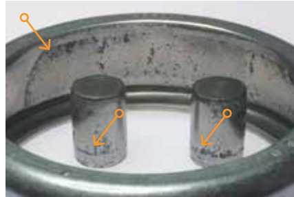
Fig. 12: Cylindrical bearing outer race and roller peeling and wear caused by underfilling.
