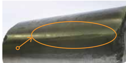
Fig. 13: Cylindrical roller flattened as a result of skidding.
