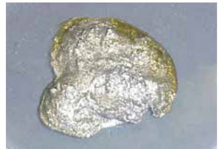
Fig. 3: Grease from an underfilled bearing contaminated with metal debris.
