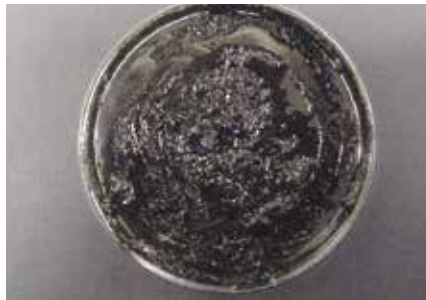
Fig. 2: Heavily oxidized grease from an overfilled bearing.
