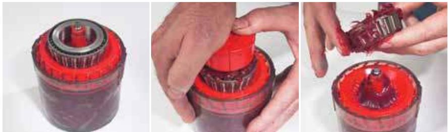
NOTE: You should allow enough space in the housing for heat dissipation so excess grease throws clear from the bearing. Contain the grease around the bearing. The housing should normally be 1/3 to 1/2 full of grease during bearing assembly. Too much grease in the housing may cause high temperatures and excess churning of the grease.
