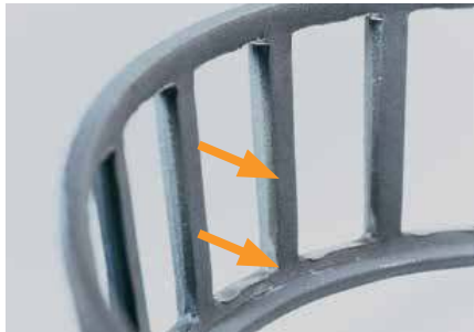
Fig. 2 – Cage pocket wear: heavy contact between the rollers and cage pocket surfaces caused by bearing operating too loosely.
