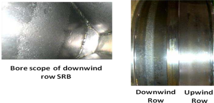
Figure 2: Early stages of SRB micropitting in a turbine mainshaft
