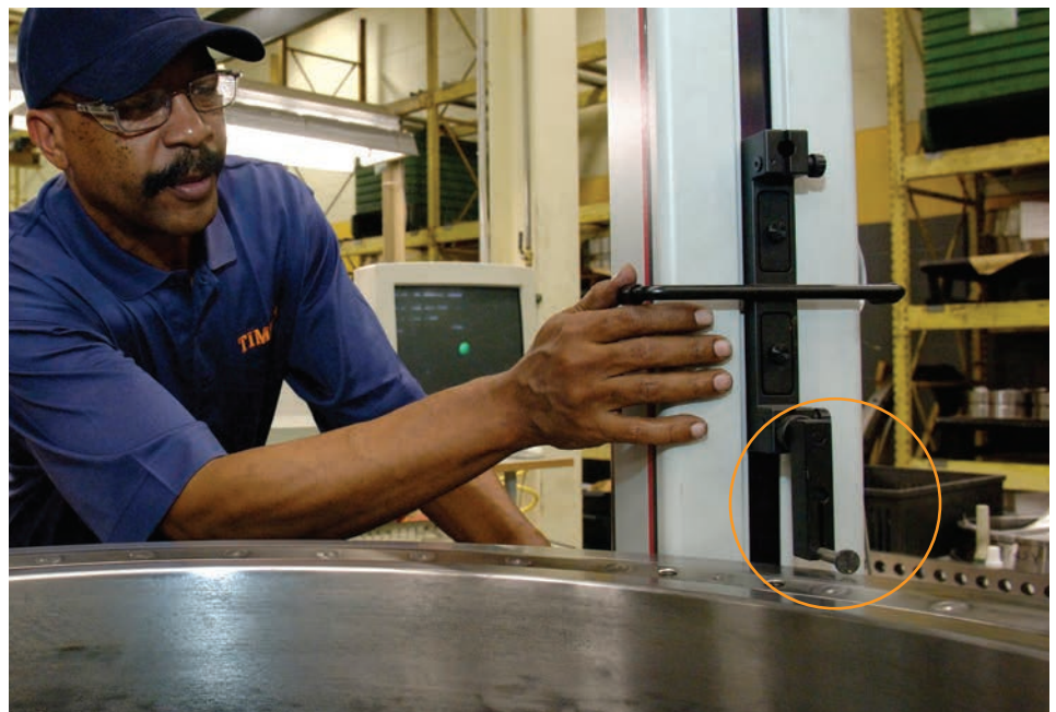
Figure 5: Timken technicians measure the bore, O.D. and width of the bearing, as well as record the roundness of the major race components to help determine the appropriate method of repair.
