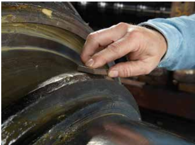
Fig. 44 Remove any burrs or sharp edges from the seal riding surface of the roll neck
