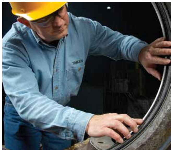
Fig. 29 Seals should be inspected and replaced if necessary
