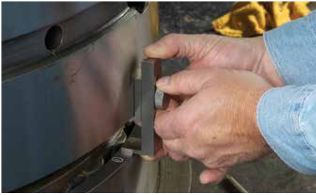
Fig. 19 Measure the B, D and C gap for wear
