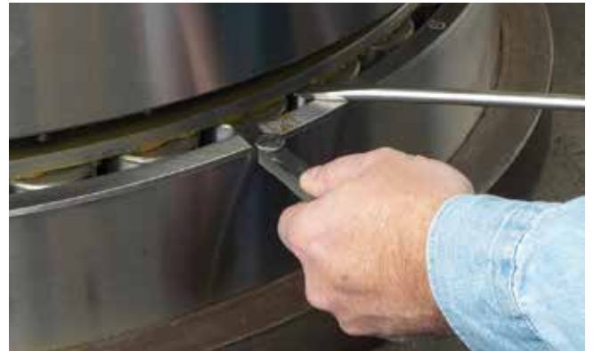
Fig. 18 Use a feeler gage to check for proper bearing seating
