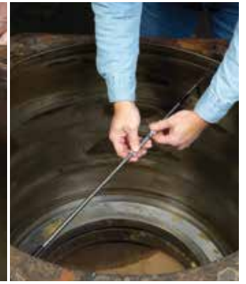
Fig. 24 Check for chock bore size and out-of-roundness
