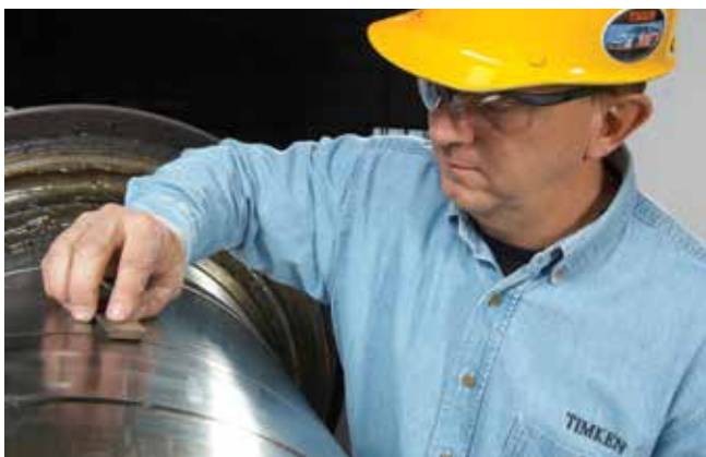
Fig. 42 Remove any nicks or gouges on the roll neck
