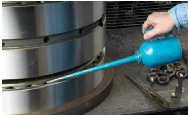
Fig. 17 Apply a light coating of oil to protect the bearing
