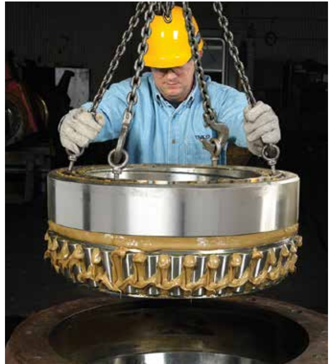
Fig. 38 The top double cone and cup are the last components to be installed into the chock
