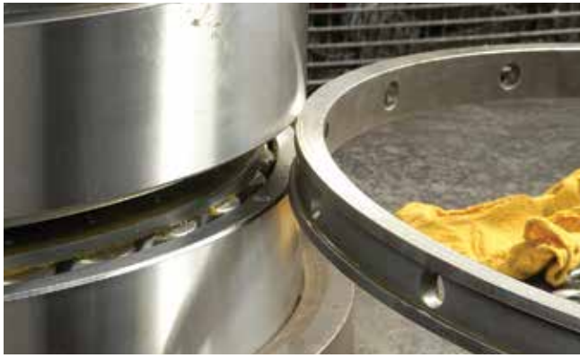
Fig. 21 With the proper bearing end play, the spacer width is greater than the spacer gap
