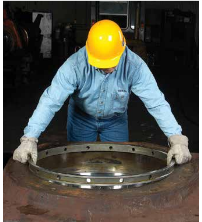
Fig. 37 Place the cone spacer and top cup spacer into position
