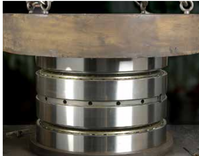
Fig. 14 Weight the bearing to properly seat components
