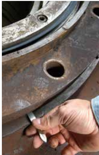
Fig. 40 Use a feeler gage to make sure the cups are properly clamped
