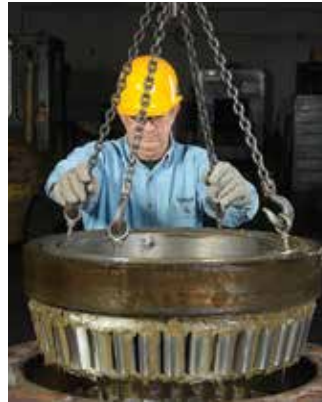
Fig. 8 Remove the top single cup and double cone
