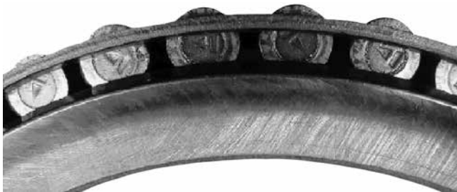
Fig. 183. Roller end and rib discoloration.
