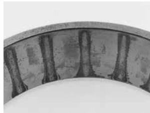
Fig. 189. Staining without pitting.
