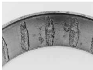
Fig. 191. Deep etching on an outer ring race.
