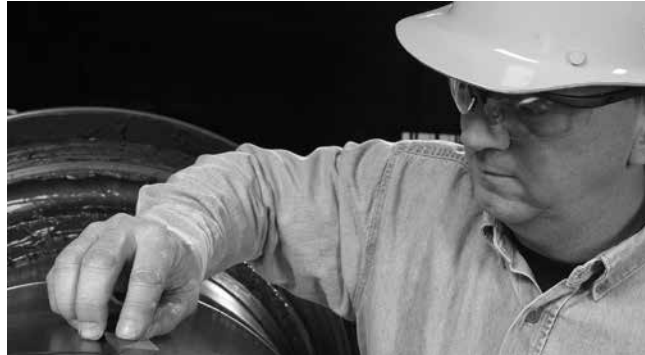
Fig. 240. Restoring minor roll neck damage.
