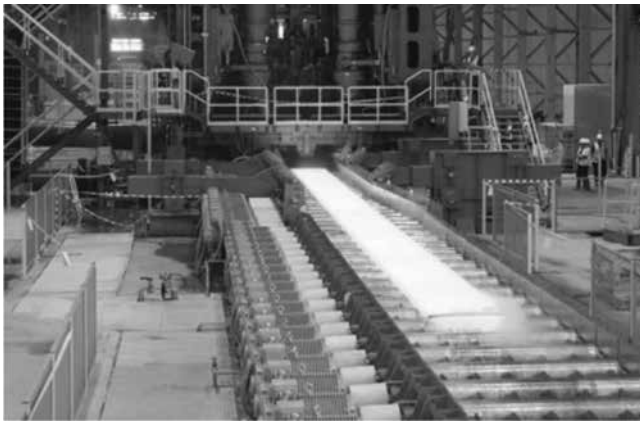
Fig. 113. Hot-strip mill transfer roller table.
