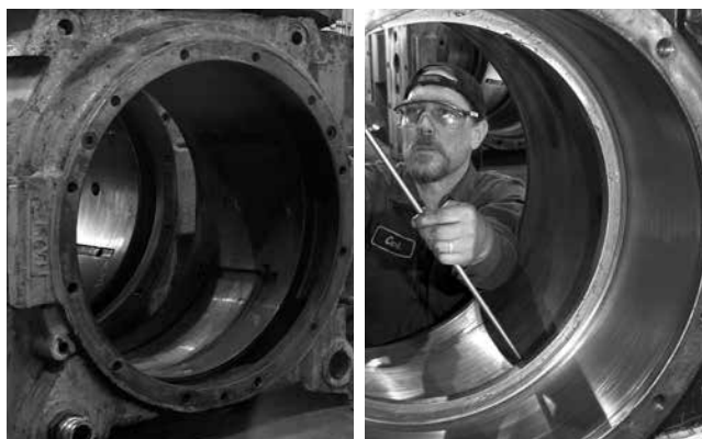
Fig. 278. Chock maintenance before and after photos.
