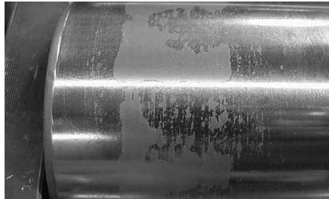
Fig. 184. Roller peeling damage.
