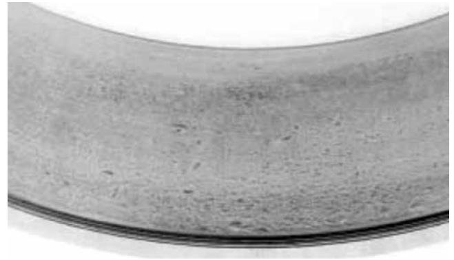
Fig. 160. Bearing damage due to abrasive particles.
