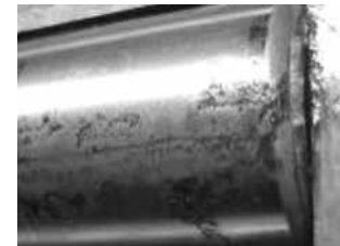
Fig. 190. Pitting on roller.
