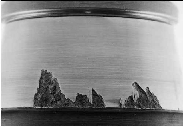
Fig. 171. Geometric stress concentration spalling.
