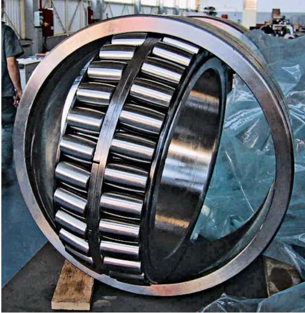
Spherical roller bearings, post bearing remanufacture.
