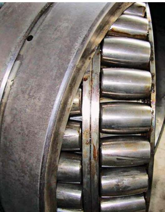
A large spherical roller bearing and outer race showing the condition of a bearing in need of bearing repair services.
