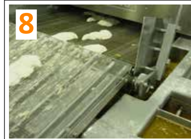
'NA' or 'FA' bearing on fryer infeed and outfeed belts (depending on temperature at bearing)
