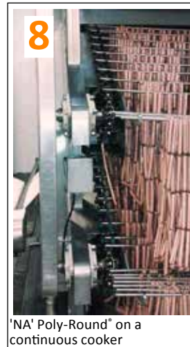
Solid lubricated ball bearings in stainless QuiKlean® with a back seal work well as EDT Breeder Bearings
