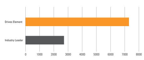
Drives Element roller chain outlasts the industry leader's sintered bushing chain by more than 2.5x. (1) ANSI 60 chain, 275 RPMs, 230 lbs. (1023N) tension, 3.0 chain horsepower (2.24 kW), 23T x 23T sprockets.
