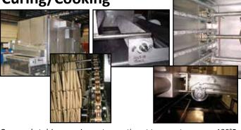
On sprocket-driven equipment operating at temperatures over 180°F (82°C) like continuous cookers, smokehouses, microwave and standard ovens, Poly-Round® bearings eliminate grease melting out of ball bearings. On belt washers, greaseless Poly-Round® bearings are also
