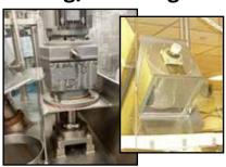
Type E Solution® bearings for large shafts (to 5" / 127mm), and Poly-Round® bearings for standard shafts (1/2" to 3" / 12.7mm to 76.2mm), are the most sanitary bearings available: no contamination, no corrosion, and no need to re-grease after washdown.
