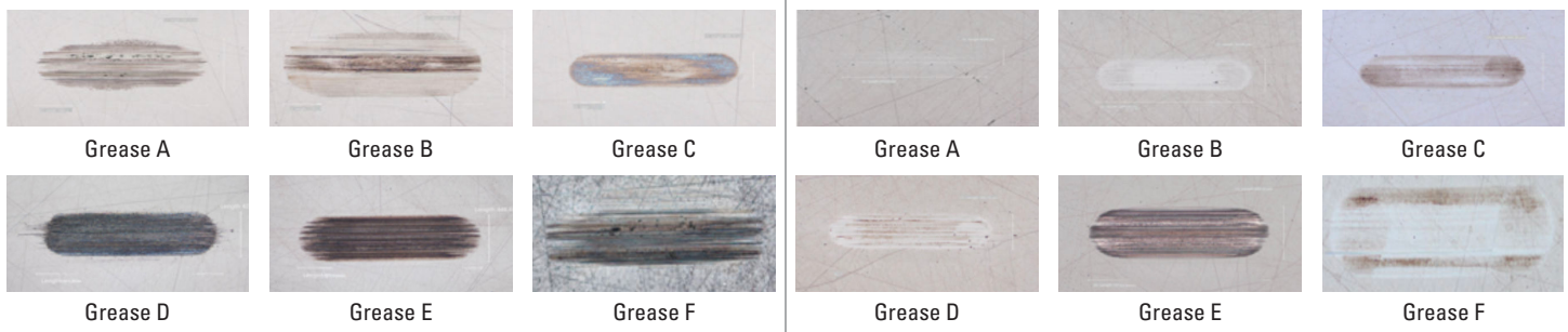
Figure 9. Fretting Wear Scars Non-DLC (left) DLC (right)
