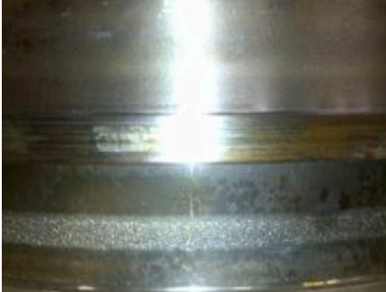
Figure 2. Micropitting on a Spherical Roller Bearing Inner Race
