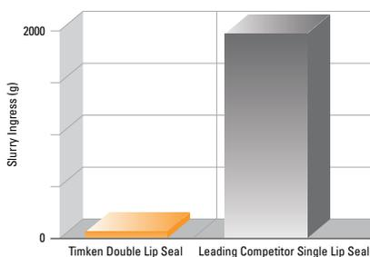
Slurry ingress test results of the Timken Type E seal compared with the R seal design of a leading competitor. Seal operating at 250 rpm in a salt and mud slurry mixture for 75 hours.
