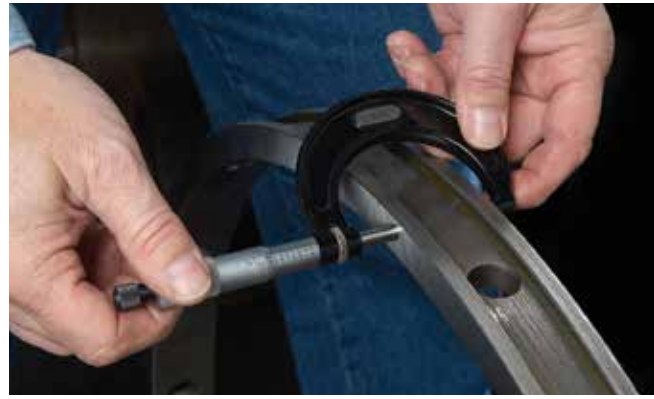
Fig. 20 Measure the B, D and C spacer width
