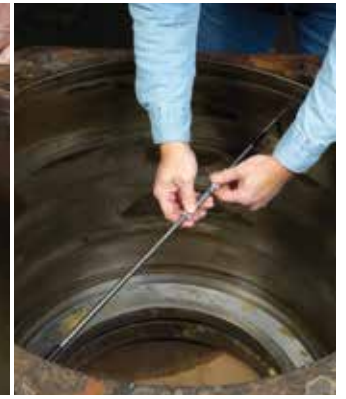
Fig. 24 Check for chock bore size and out-of-roundness
