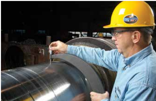
Fig. 41 Before mounting the bearing, check the roll neck for size
