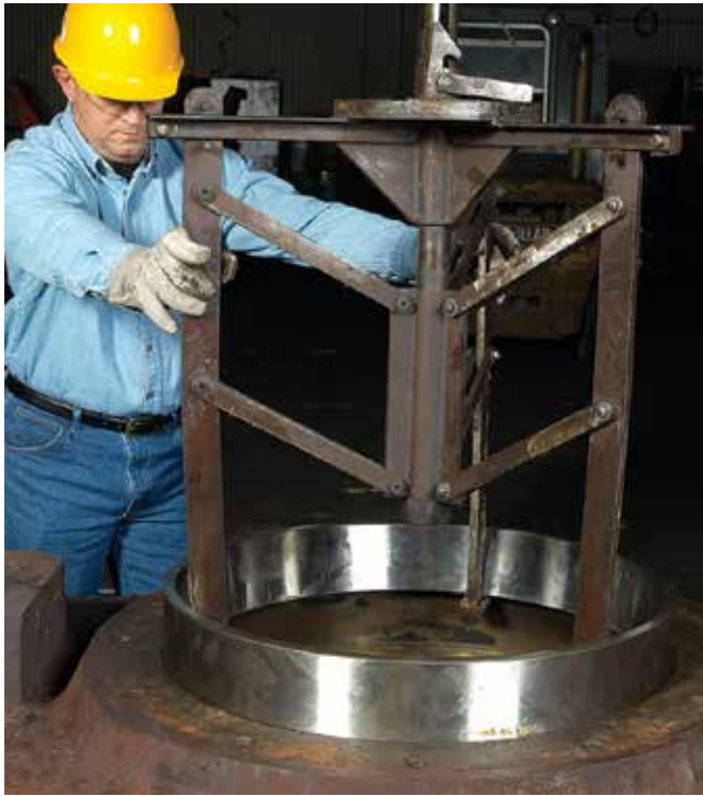
Fig. 33 Install the bottom cup into the chock
