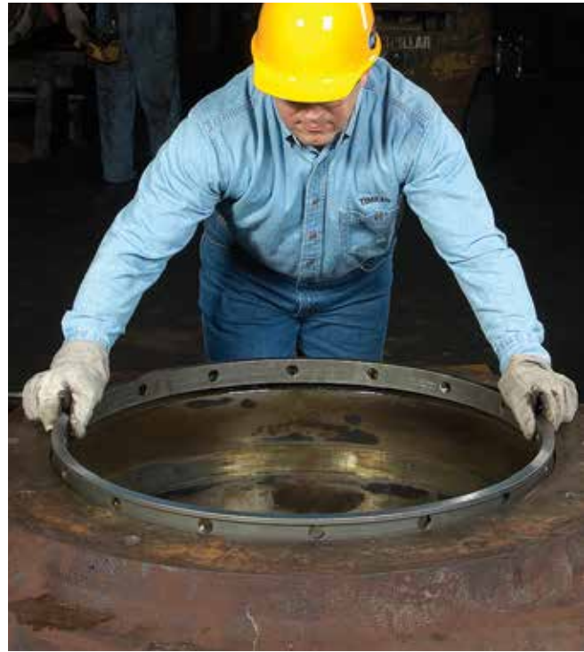
Fig. 34 Install the cup spacer
