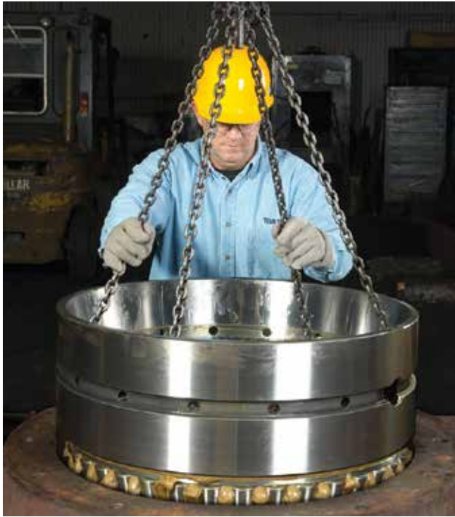
Fig. 36 Install the bottom double cone and double cup into the chock
