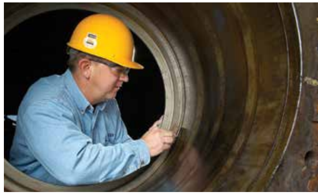
Fig. 27 Remove any nicks or burrs from the chock backing shoulder
