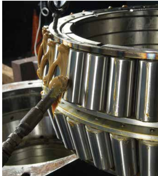
Fig. 35 Lubricate the bearing with grease
