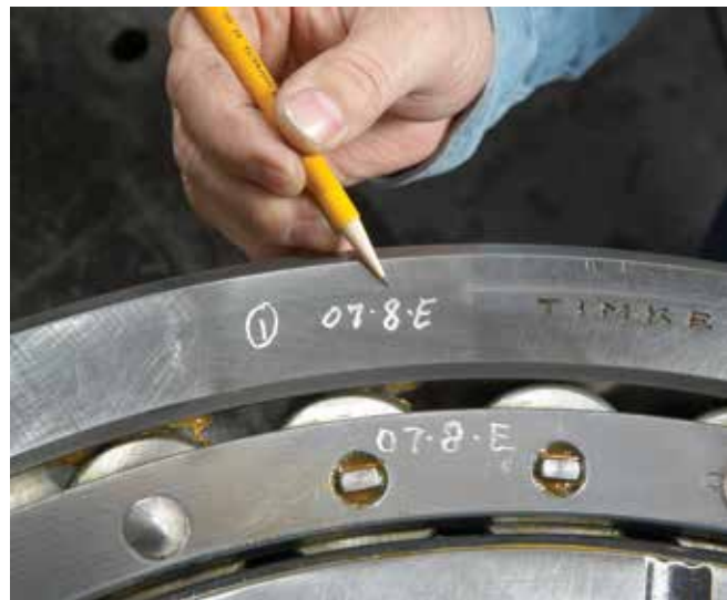
Fig. 15 Follow the Timken lettering system to ensure proper stacking order
