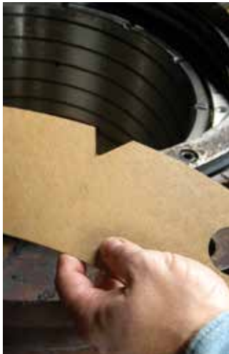
Fig. 39 Notch the gasket
