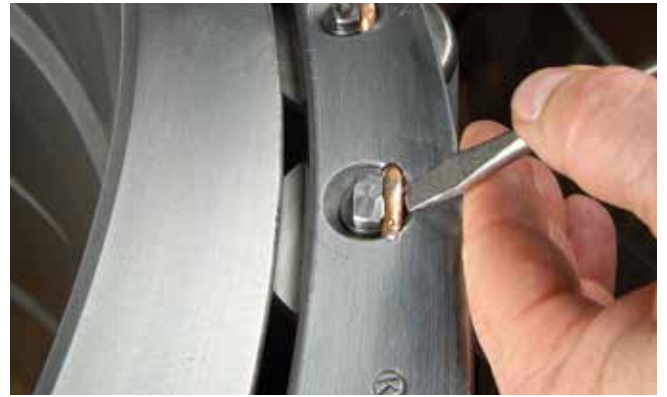
Fig. 11 Remove the pin locking wire
