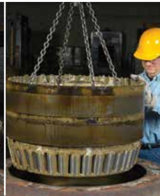
Fig. 9 Remove the double cup, bottom double cone, cone spacer and top cup spacer
