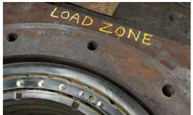
Fig. 32 The load zone in a back-up roll chock
