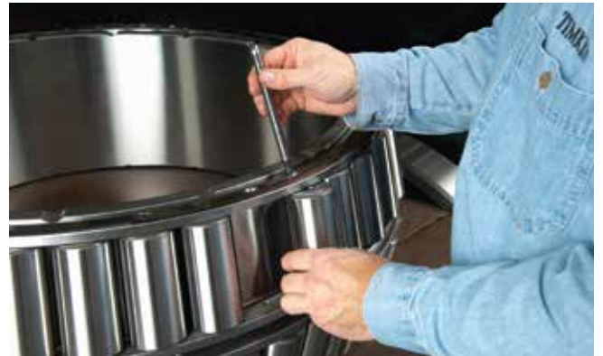
Fig. 12 Remove the roller to inspect the bearing raceway for damage
