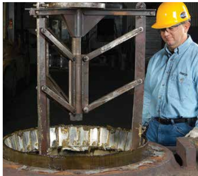
Fig. 10 Remove the bottom single cup and cup spacer
