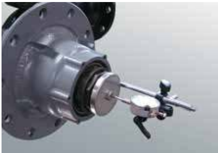
Fig. 3 – A typical end play gauge.
