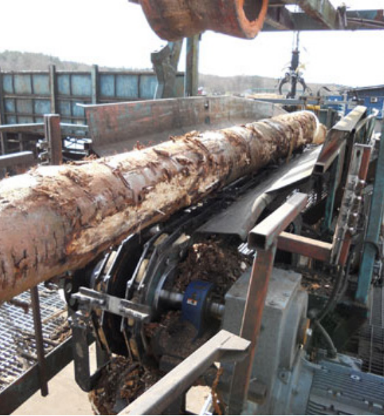
Figure 2: In a Derome Timber sawmill in Sweden, Timken pedestal roller bearings with a solid housing achieved a service life more than four times longer than that of previously used bearings units with a cast iron housing.
