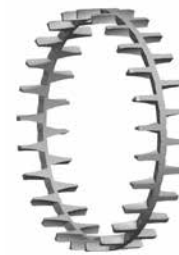
Fig. 45. One-piece, machined-brass, land-riding, finger-type cage.
