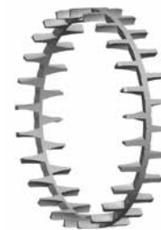
Fig. 45. One-piece, machined-brass, land-riding, finger-type cage.
