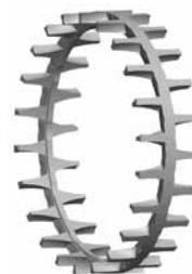
Fig. 44. One-piece, machined-brass, roller-riding, finger-type cage.
