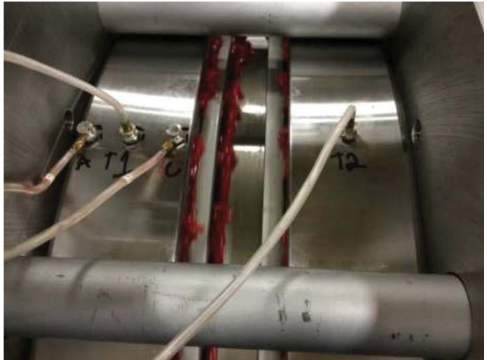
Figure 9: Location of thermocouples on cup outside diameter
