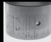
Etching and corrosion
