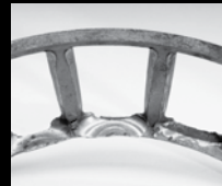
Cage pocket wear from excessive roller movement
