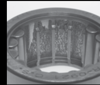
Geometric Stress Concentration (GSC) spalling on outer ring
