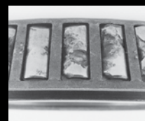
Severely fatigued rollers from heavy load
