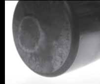
Roller end with adhesive wear
