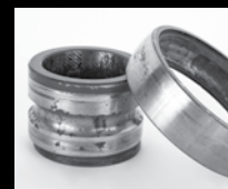
Advanced corrosion and etching
