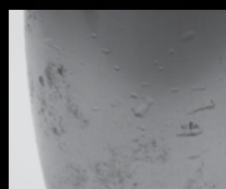
Hard particle contamination
