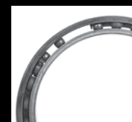
Cage damage from bearing lockup
