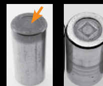
Rib and roller end heat damage
