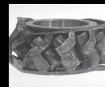
Cage damage from bearing lockup
