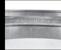
Burns from electric current
