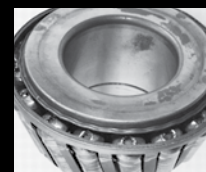
Race deformation from excessive heat generation
