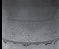
Spherical roller bearing with adhesive wear
