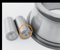
Fine particle contamination
