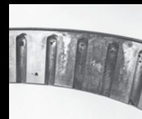
Heavy false brinell on outer race
