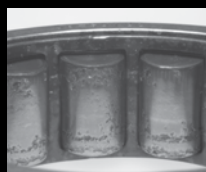
Fatigue resulting from heavy loads
