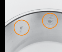
Roller spaced nicking
