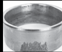
Geometric Stress Concentration (GSC) spalling on inner ring
