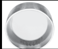
Elliptical roller path caused by misalignment
