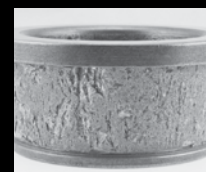
Severe peeling and spalling from heavy loads
