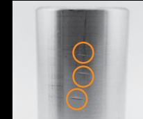
Nicks and dents caused by rough handling
