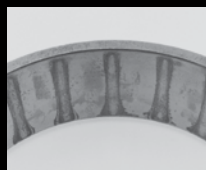
Light corrosion on the outer race
