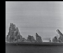
Geometric Stress Concentration (GSC) spalling
