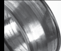
Adhesive wear on bearing inner ring
