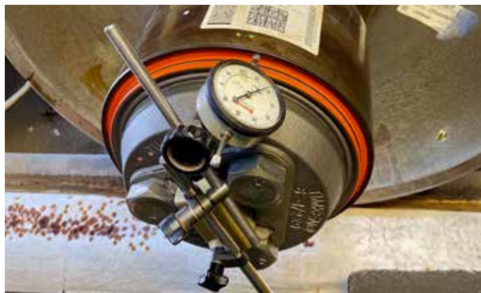
Fig. 13. Checking mounted lateral.
