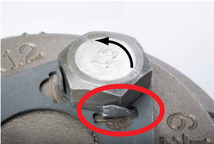
Fig. 11. Shows INCORRECT position. This position will not resist loosening (the arrow indicates loosening direction of the cap screw).
