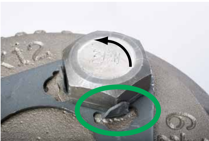
Fig. 12. Correct position of tab against cap screw head flat. This position helps resist loosening of the cap screw (the arrow indicates loosening direction of the cap screw.).
