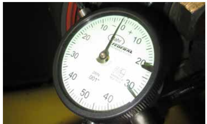
Fig. 14. The bearing lateral endplay should be 0.001 in. to 0.015 in. (Amtrak 0.001 in. to 0.020 in.).
