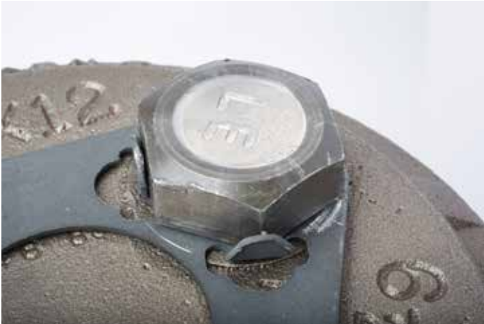
Fig. 10. If cap screw head is centered on a locking plate tab, see figures 11 and 12 below.
