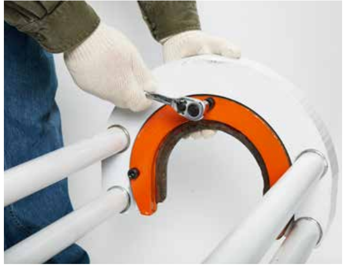
Fig. 17. Ensure the pulling shoe adapter is securely seated inside the pulling shoe.
