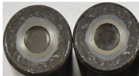
Severe Roller End Scoring Damage
