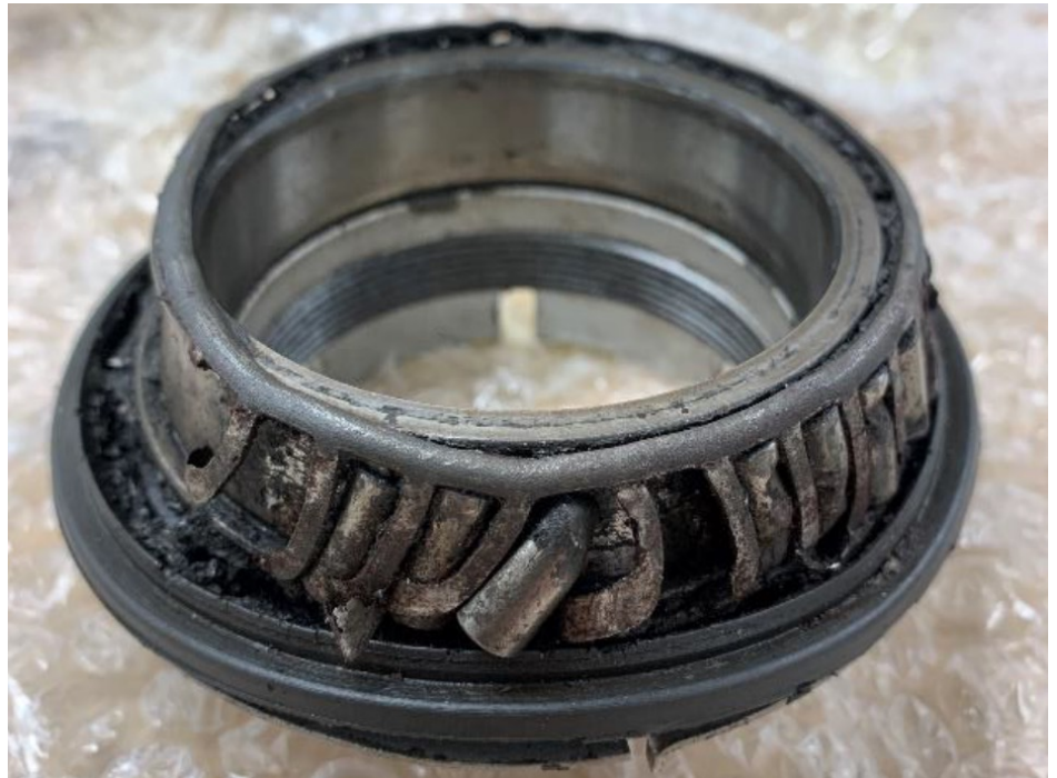
Locked Up Tapered Roller Bearing Cone Assembly
