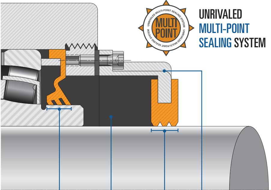
Triple lip internal seal (rubber, viton, or urethane)    Full grease pack in cover (all covers have grease zerks)    Triple lip external rubber through shaft seal\*    External through shaft cover (urethane or steel)
