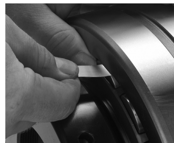
Fig. 18. Measure RIC before installation.
