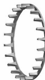
Fig. 7. YMD Split, machined-brass, land-riding, finger-type cage.
