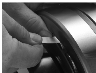
Fig. 14. Measure RIC before installation.
