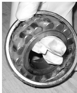
Fig. 21. Grease can easily be packed by hand.
