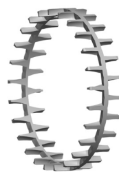
Fig. 5. EM/YM One-piece, machined-brass, roller-riding, finger-type cage.
