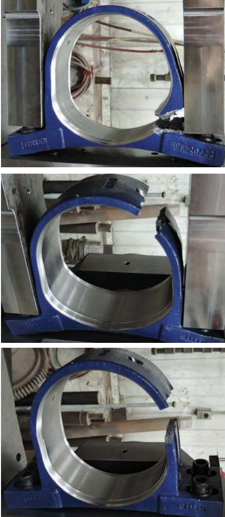
Figure 4: Fracture of split housings.
