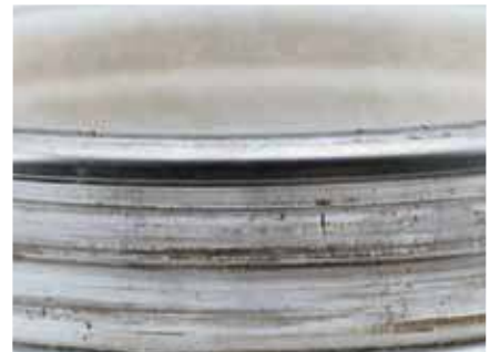
Bearing cup (outer race) damage caused by an excessively loose fit in a rotating hub.
