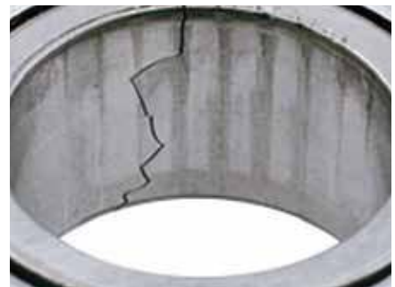
Bearing cone (inner race) bore damage - Fractured inner race cause by out-of-round or oversized shaft.
