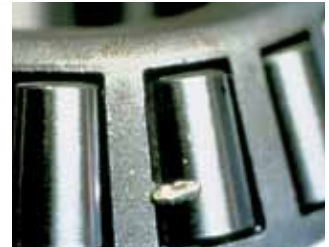
Grooving: Large particle contamination embedding into soft cage material.
