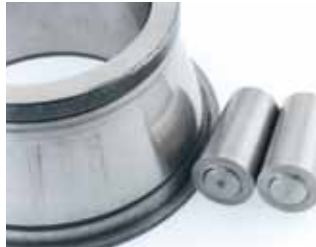
Abrasive wear: Fine abrasive particle contamination.
