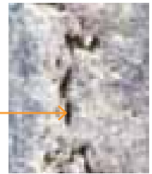
Fluting: Series of axial burns caused by electric current passing through the bearing while rotating.
