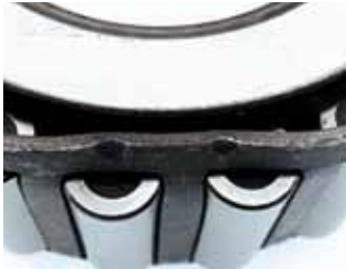
Cage deformation: Improperly installed or dropped bearing.
