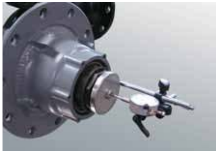
Fig. 3 – A typical end play gauge.
