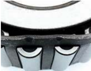
Cage deformation: Improperly installed or dropped bearing.
