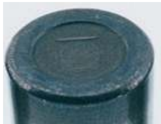
Bearing cone (inner race) large rib face scoring: 'Welding' and heat damage from metal-to-metal contact.
