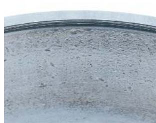
Bruising: Debris from other fatigued parts, inadequate sealing or poor maintenance.
