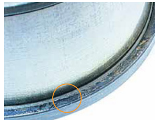
Bearing cone (inner race) large rib face scoring: 'Welding' and heat damage from metal-to-metal contact.
