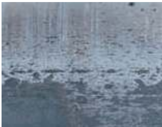
Micro-spalling due to thin lubricant film from high loads and low RPM or elevated temperatures.
