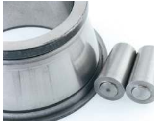
Abrasive wear: Fine abrasive particle contamination.
