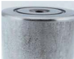
Micro-spalling due to thin lubricant film from high loads and low RPM or elevated temperatures.
