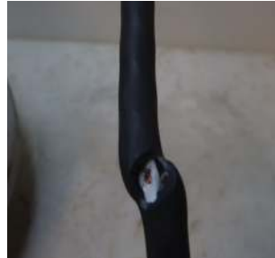
Avoid pinched cable by using retainer clips.
