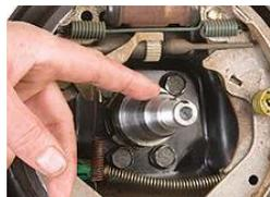
mineral spirits. Inspect the spindle for wear. Use a fine file, wire brush, emery cloth or honing stone to remove any debris, nicks or burrs. Follow the vehicle manufacturer's recommendation for permissible spindle wear. Apply a light grease coating on the cone seats to ease installation and prevent fretting.
