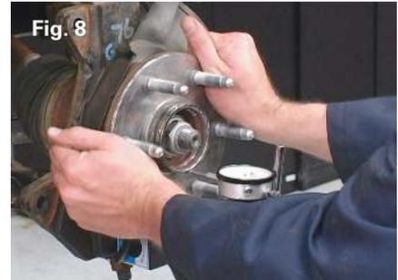
10. Observe the total indicator movement. If it exceeds 0.004", replace the hub bearing assembly. (Fig. 9)
