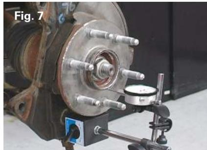
9. Grasp the wheel flange at the 3 and 9 o'clock positions, and push while oscillating the hub bearing assembly approximately 90° side-to-side at least five times. Set the dial indicator to zero. Next, pull while oscillating the hub bearing assembly approximately 90 degrees side-to-side at least five times. Proper loading and oscillation is necessary to fully seat the bearings. (Fig. 8)
