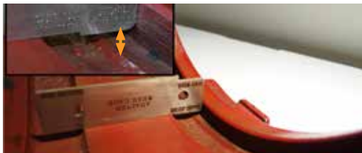
Arrows indicate an acceptable space between the toe of the gage and the machined relief of the adapter.
