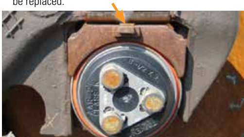
Acceptable adapter: relief is not in contact with the roof liner
