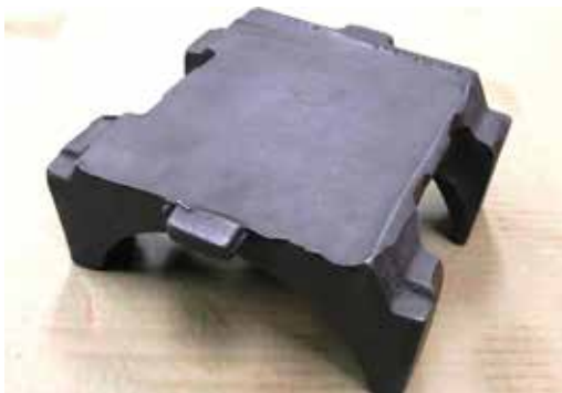
Adapter with excessive wear
