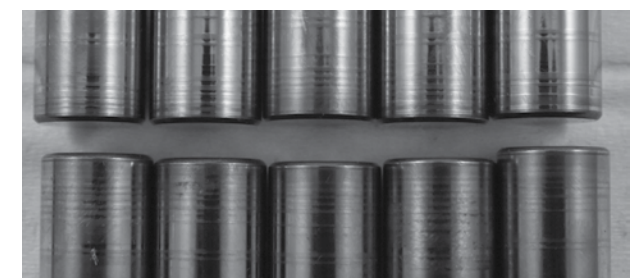
Circumferential grooving on rollers
