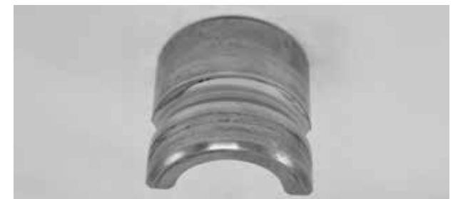
Elliptical wear path on inner ring
