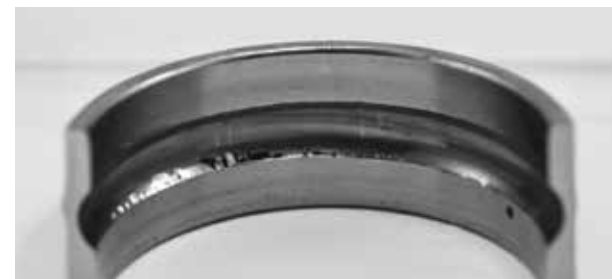
Spalling at outer race edge
