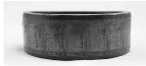
Roller spaced corrosion etching
