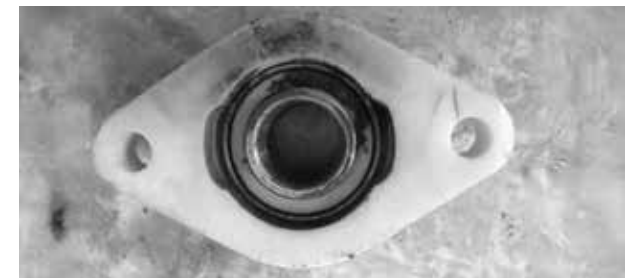
Chemical reaction with lubricant
