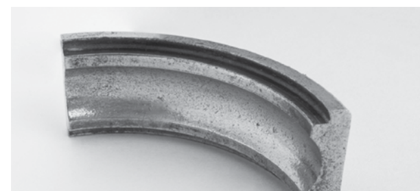
Dented outer raceway
