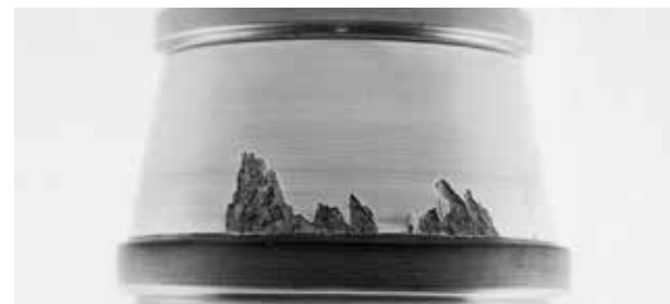
Geometric Stress Concentration (GSC) spalling on inner ring
