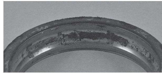
Corrosion on outer ring raceway and shoulder
