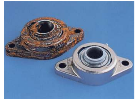
The Survivor unit outperformed other designs in demanding salt spray tests.
